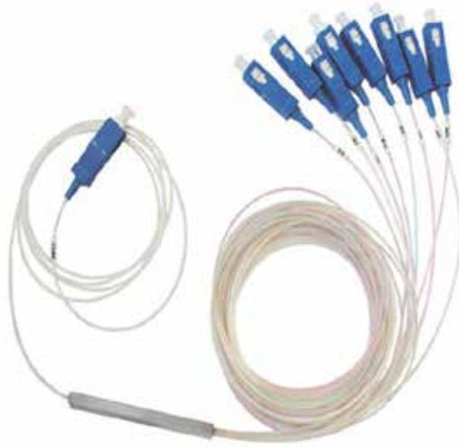
1x8 Fiber PLC Splitter Singlemode G.657A1 fiber, 900µm input/output, 1260-1650nm, mainly used in 8,16 cores optical distribution box
