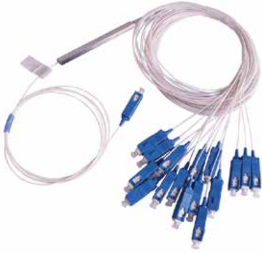
PLC Splitters 1x16 Single mode with Corning SMF-28e fiber cable & SC/APC, SC/UPC, FC, LC Connectors
